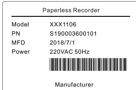
**Notice:** Please check the power specifications according to the order model and make sure that the type of power supply is 220V AC or 24V DC in order to avoid damaging the instrument.
