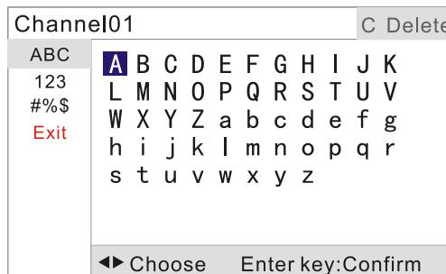
The input method is used in text editing. On the left, [up and down keys] switch the classification and alphabet, on the right, [left and right keys] move the text cursor, [confirmation keys] select the text, [Cancel C keys] delete the text.
