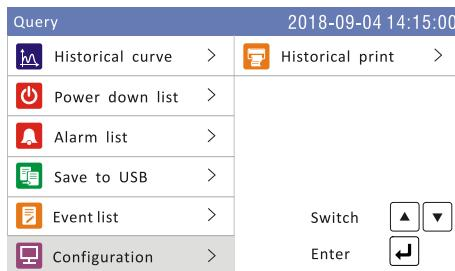
Enter the password, press [Enter key] to enter the configuration interface, the initial password is 0000.
